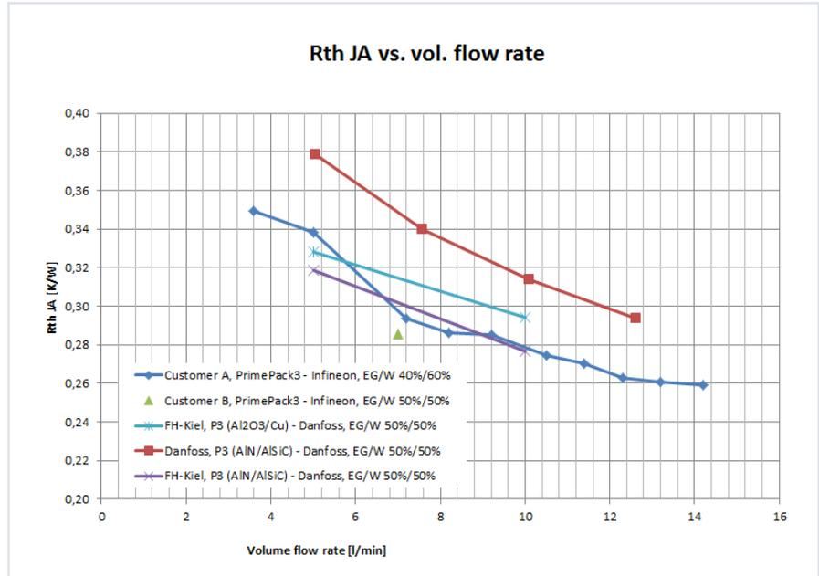
Thermal resistance, junction-water, for one single IGBT chip in the P3 module.
