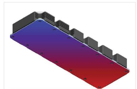
Temperature gradient in standard cooler.
